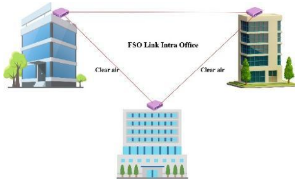
Figure 2. Illustration of Intra-Office FSO Link Scenario
