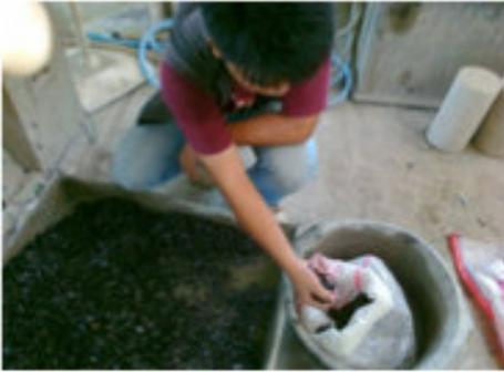
Gambar 4. Proses Pencucian Agregat
