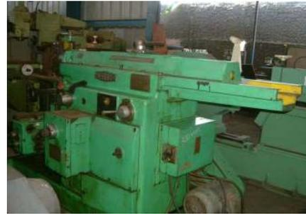
Gambar 7. Mesin Skrap (*Shaping Machine*)
