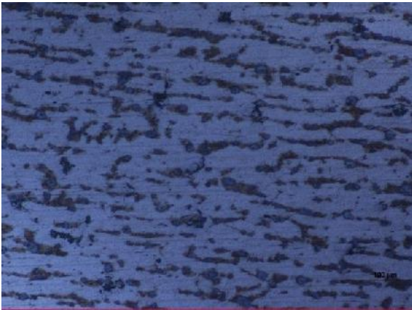
Gambar Base (Proses Perlakuan Panas 650 0 c)
