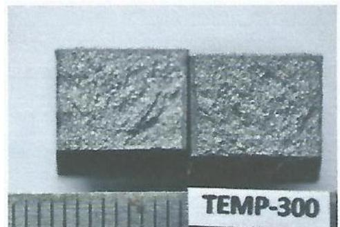
Gambar 4.3 Penampang patah tempering 300°C
