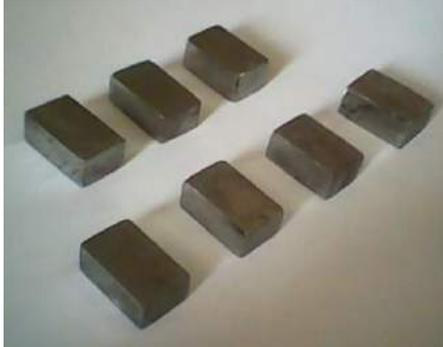
**Gambar 3.4 Specimen Baja Hardox 400**
